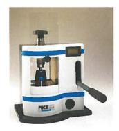
Place the die with loaded sample in the pellet press. Attach to the vacuum line and start pulling vacuum to remove moisture, about 1 to 2 minutes. Compress the die to a maximum of 10 tons. Wait for 1 minute minimum; although press time and pellet quality are a function of pellet thickness and applied pressure and time may vary for optimal results. Release the pressure and remove the die from the press.
