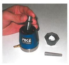
Place piston in the well of the block assembly. The O-ring provides support for the piston and it seals the gap between the piston and the barrel when vacuum is applied.
