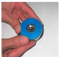
Turn the die upside down and remove the base. Place the piston on a hard surface and press. The pressure should push anvils and the pellet toward you. If hand pressure is insufficient, tap gently with a hard object, until the assembly releases.
