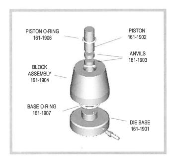
The PIKE Evacuable KBr Die Kit features the following components: a stainless steel base with vacuum outlet, the main die block with a 13-mm cylinder, two anvils, a plunger, and an ejector ring. Components are made of hardened stainless steel, and surfaces that come in contact with the sample are highly polished. Two different size O-rings are used to seal the base/die assembly and the plunger.
