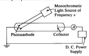
In this apparatus, the photocathode and the collector are made from the same material. The potential V of the collector, measured relative to ground, is initially zero and is then increased or decreased monotonically. The effect is described by Einstein's photoelectric equation
