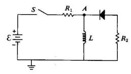
94. In the circuit shown above,  $R_2 = 3R_1$  and the battery of emf  $\mathcal{E}$  has negligible internal resistance. The resistance of the diode when it allows current to pass through it is also negligible. At time t = 0, the switch S is closed and the currents and voltages are allowed to reach their asymptotic values. Then at time  $t_1$ , the switch is opened. Which of the following curves most nearly represents the potential at point A as a function of time t?
