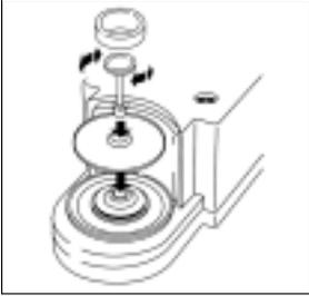
● Place the components listed below on the weighing cell (35) one at a time in the order given:
