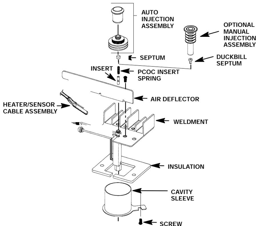
7. Remove the air deflector using a Pozidriv screwdriver to remove the screw securing the air deflector to the inlet weldment.
