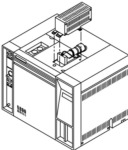
8. Remove the extension spring holding the PMT assembly to the support bracket.
