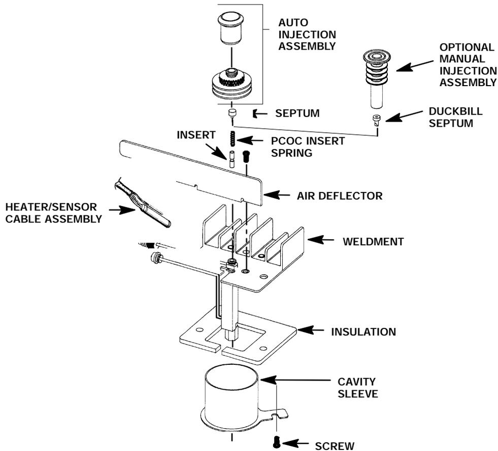
13. Remove the air deflector using a Pozidriv screwdriver to remove the screw securing the air deflector to the inlet weldment.
