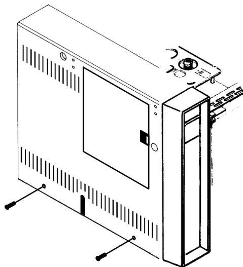
9. Remove two nuts securing the flow module to the mainframe (one next to the pressure gauge and one at the lower edge of the module).
