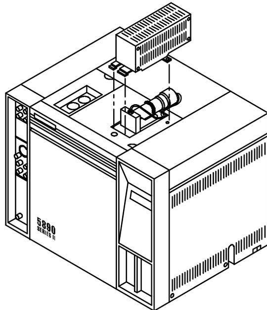
6. If an autosampler is installed on the instrument, it will be necessary to remove it and its mounting bracket to allow removal of the left side cover as follows:
