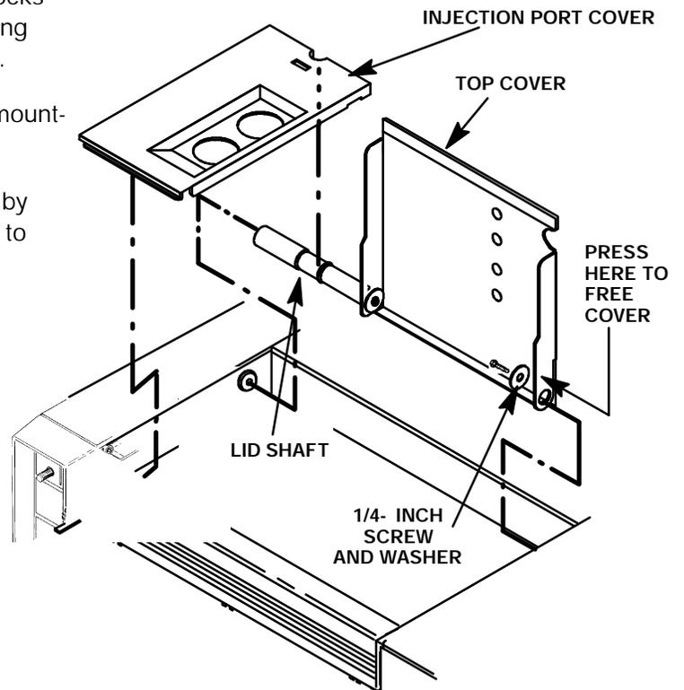
5. Remove the electronics carrier top cover .
