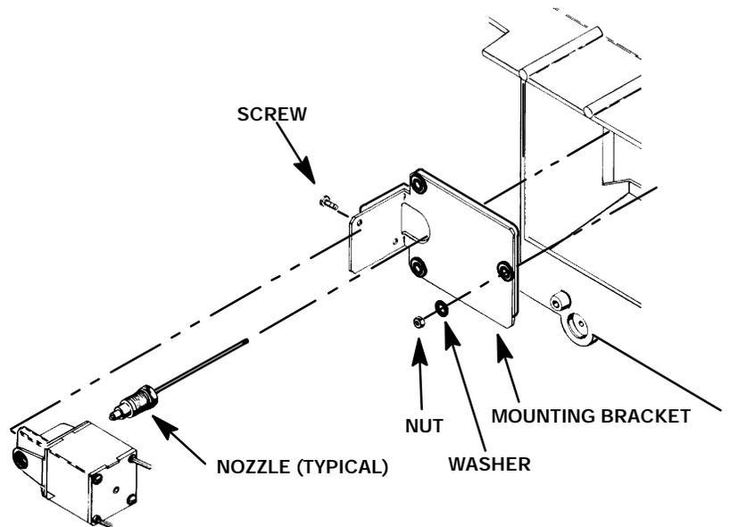
17. Withdraw the valve assembly from the side of the instrument, being careful not to bend or damage the nozzle assembly.
