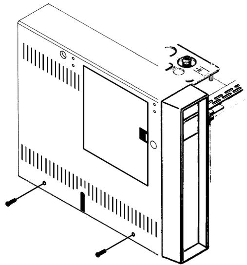
11. Lift the hinged top cover at its front edge, exposing the detector area.
