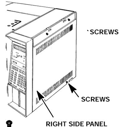
16. Remove the right side panel by removing four screws: two each along its top and bottom edges.
