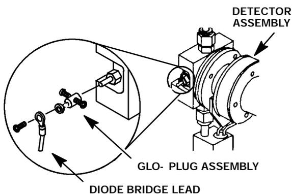
16. Trace the lead, freeing it along its path, to the diode bridge assembly.
