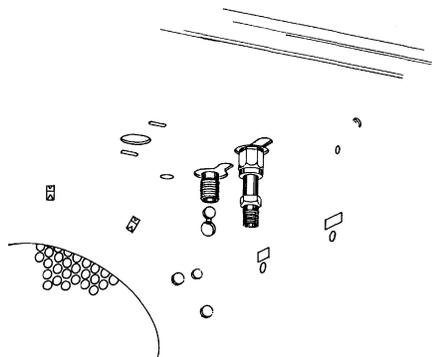
6. If the detector is not going to be replaced with a new detector, cap the detector base.
