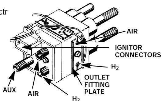
12. With a Pozidriv screwdriver, remove the mounting screw from the rear of the block. (The block must be removed from the rear of the instrument.)
