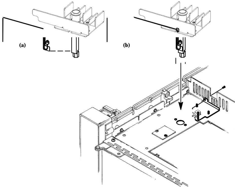
23. Install the replacement cryo- blast weldment onto the inlet weldment.
