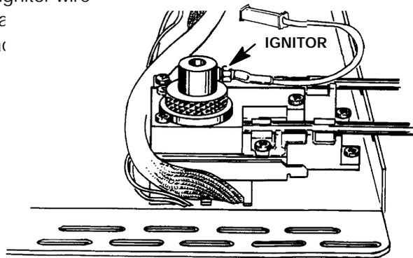
18. Loosen the screws securing the clamps holding the interconnect in place.
