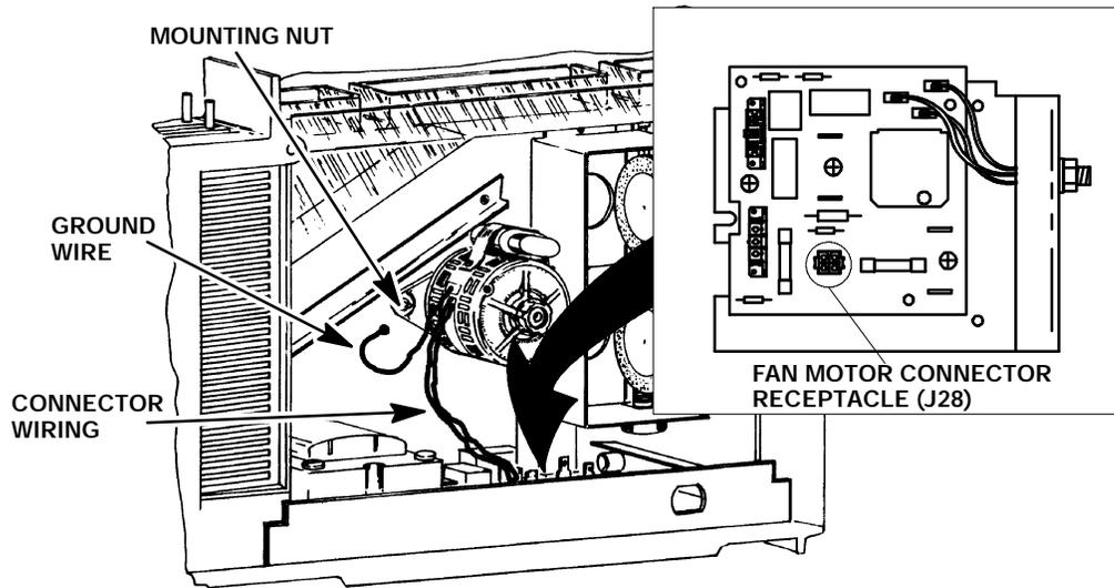
17. Remove the oven fan motor from the instrument.
