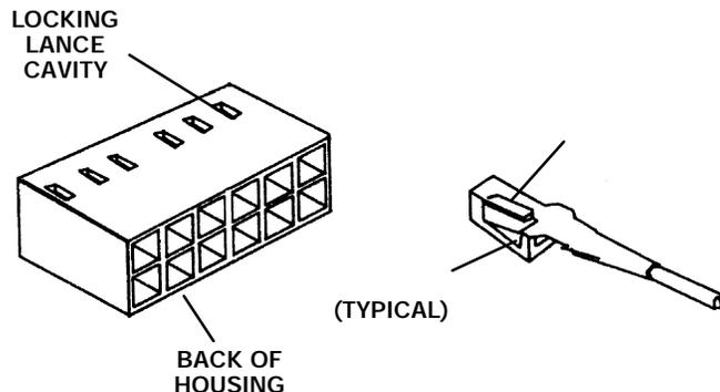
23. Gently pull on the wire to ensure that the pin is locked in the connector.
