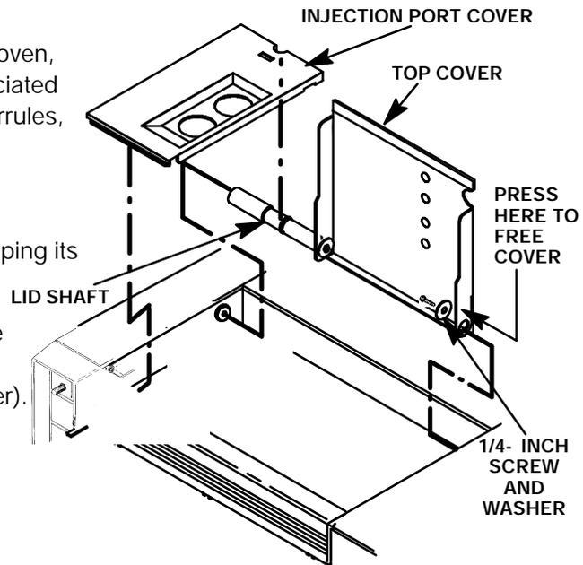
6. Use a Pozidriv screwdriver to remove the two screws securing the top cover to the instrument.
