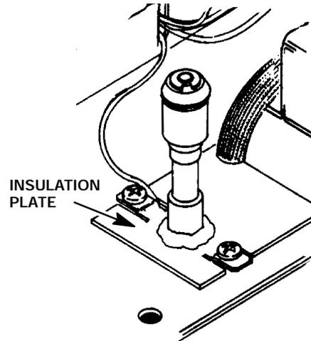
13. Lift the inlet enough to expose the heated block and heater/sensor wiring.
