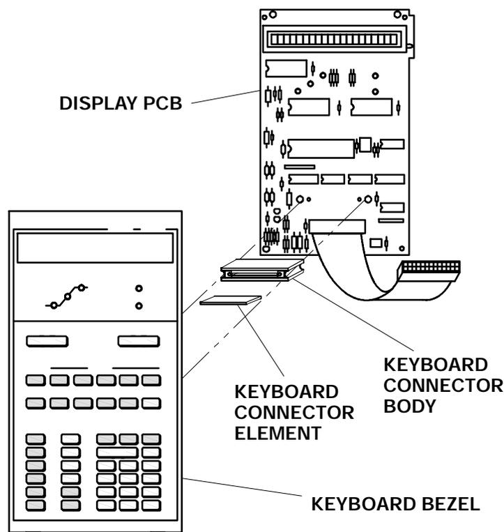
14. Install the display PCB onto the keyboard bezel (making sure that the keyboard connector element and keyboard connector body are properly installed) and secure using four screws.
