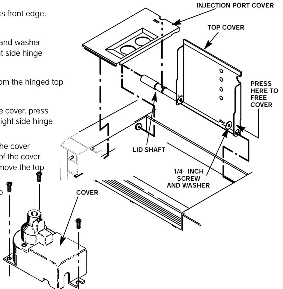
10. Remove the detector top cover, and all attached components, from the thermal strap and set aside.
