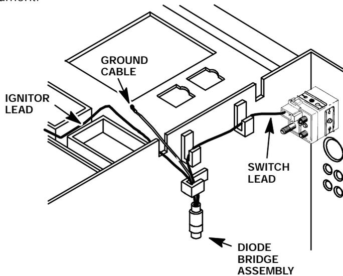
14. Install the replacement diode bridge assembly into the instrument.
