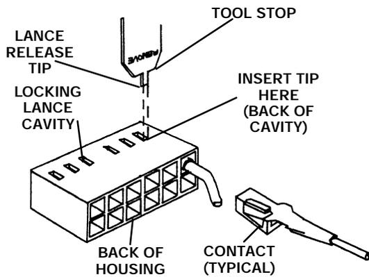
21. Prepare the pins corresponding to the replacement sensor cartridges by adjusting their locking lances using the lance reset portion of the tool.
