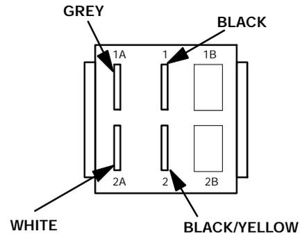
22. Install the power switch in its mounting slot (below the main PCB).
