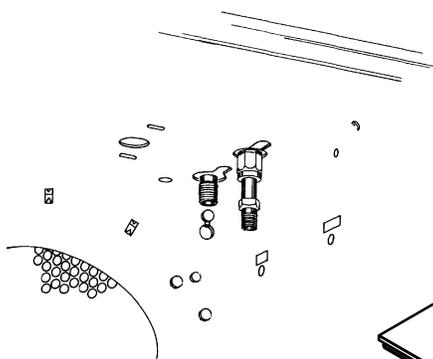
6. Remove the injection port cover by grasping its back edge and lifting it upward.
