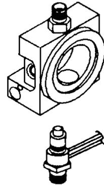
25. Insert the eraser end of a pencil (or other suitable device) through the jet opening, at the base of the detector weldment, and force the first heat shield window out of the detector weldment.
