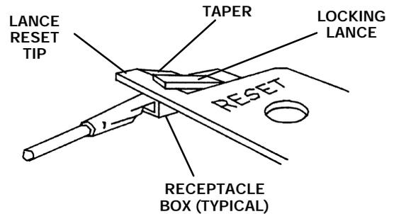
24. Insert the pins for the replacement sensor into their appropriate locations in the plug, making sure the locking lance on each pin seats into its hole through the side of the plug.
