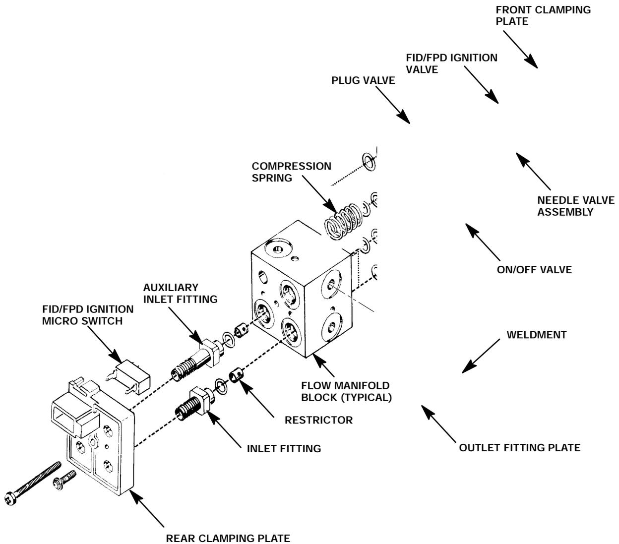
13. Install the new block on the flow panel from the rear of the instrument. The block fits on the panel over two standoffs, in only one direction.
