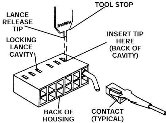
23. Prepare the pins corresponding to the replacement sensor cartridges by adjusting their locking lances using the lance reset portion of the tool.
