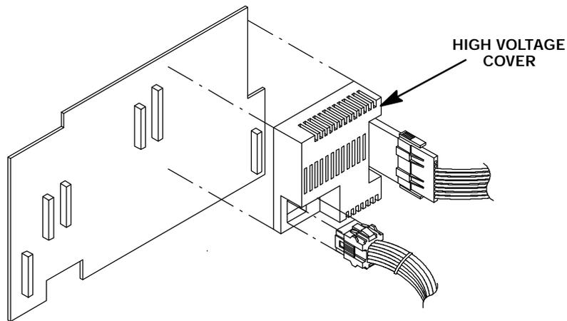
11. Disconnect connector from receptacle J9 by squeezing its ribbed sides while pulling it straight out.
