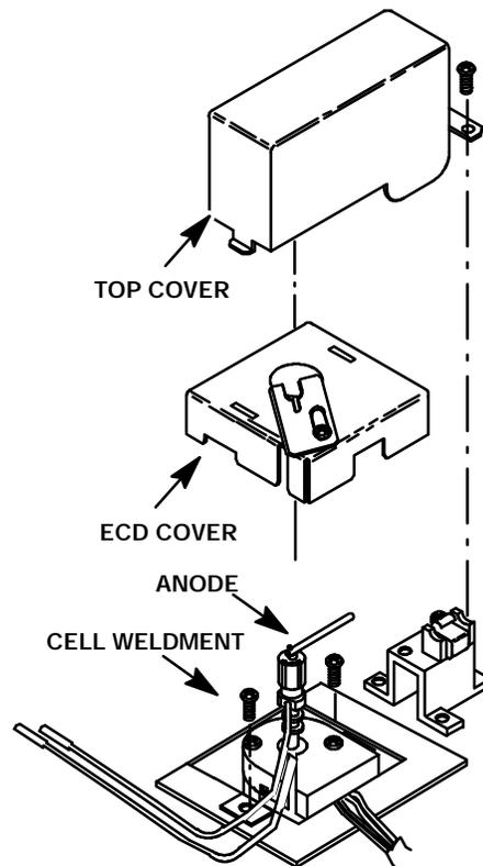
12. Loosen the anode retaining nut on the cell weldment.
