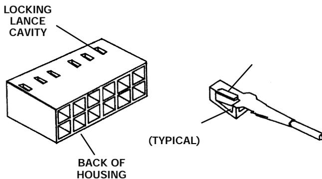
25. Gently pull on the wire to ensure that the pin is locked in the connector.
