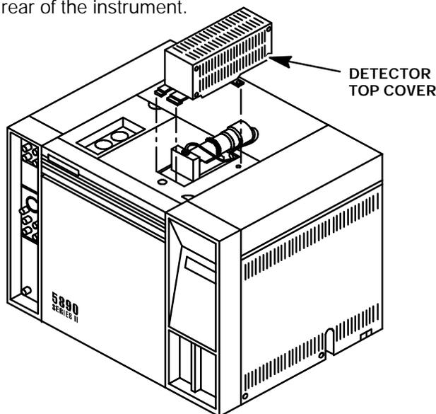
8. Lift the detector top cover to expose the FPD detector weldment.
