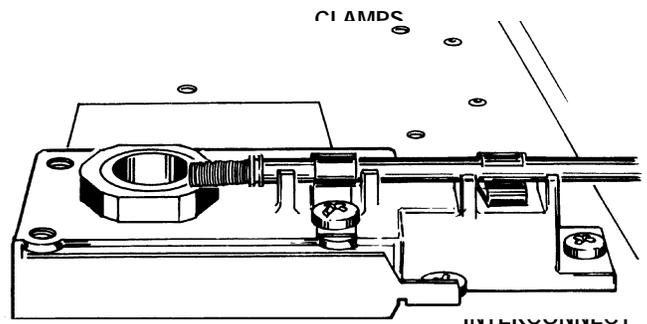
32. Tighten the screws on the clamps which secure the interconnect to the thermal strap.
