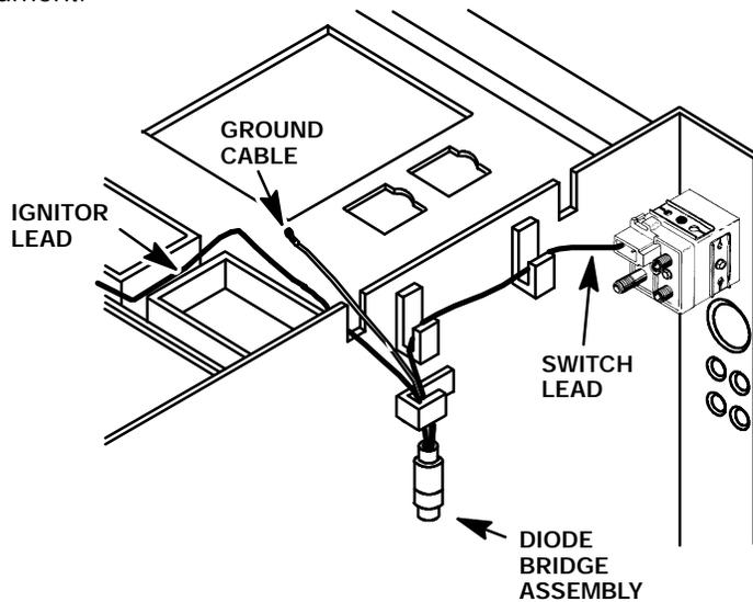
20. Install the replacement diode bridge assembly into the instrument.
