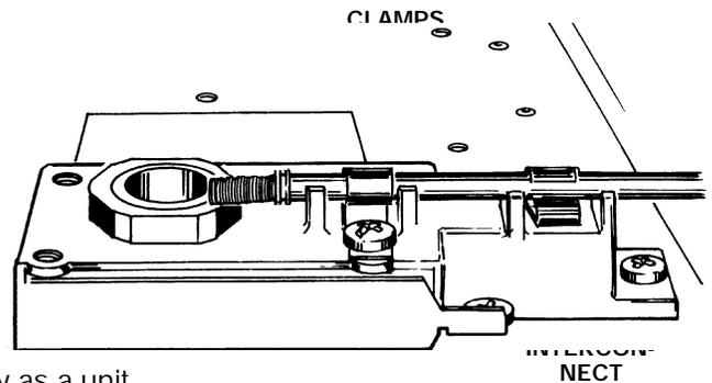
21. Tighten the screws on the clamps which secure the interconnect to the thermal strap.
