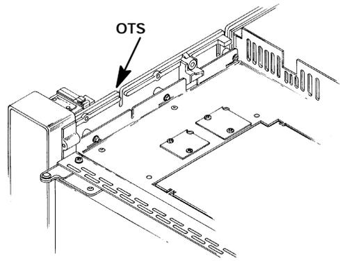
34. Connect the tubes from the new jet weldment to the flow manifold block. (The hydrogen tube fitting is painted RED. Make sure each tube is installed at the correct location on the flow manifold block.)
