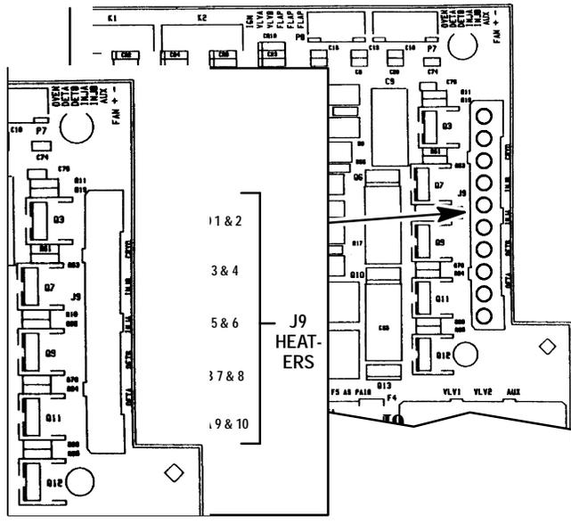
24. An AMP pin extraction tool (8710- 0614) is required to properly remove pins from connector J9. The tool features a sleeve to release the pin locking lance, and a plunger to eject the pin from the plug. The following steps detail how to remove the pins from the connector.
