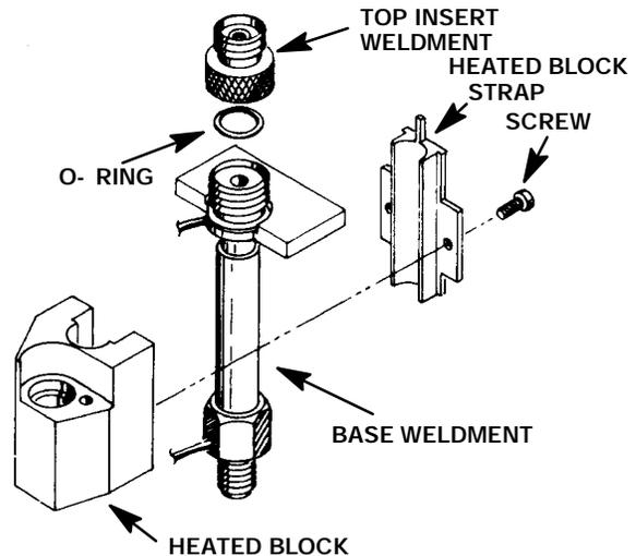
23. Carefully install the inlet into its inlet opening in the top of the instrument.
