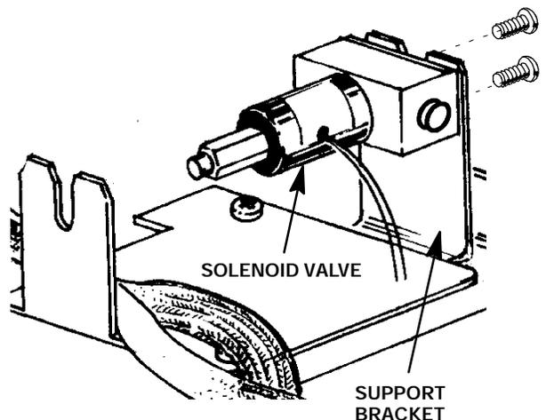
17. Install the new solenoid valve body on the mounting bracket in the same location and position as the old one.
