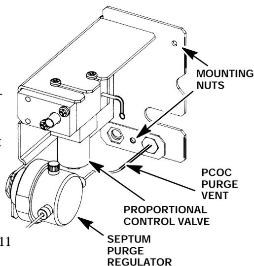
13. Remove the nut securing the PCOC purge regulator to the EPC flow bracket.
