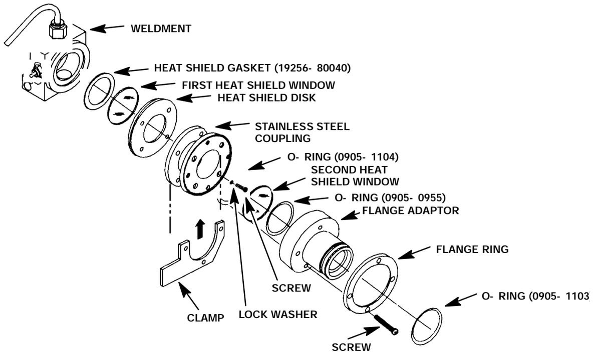
21. Remove the flange adapter and flange ring by removing the four screws securing them to the stainless steel coupling.
