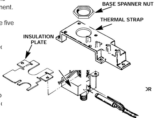
17. Slide the insulation plate out from over the detector weldment.
