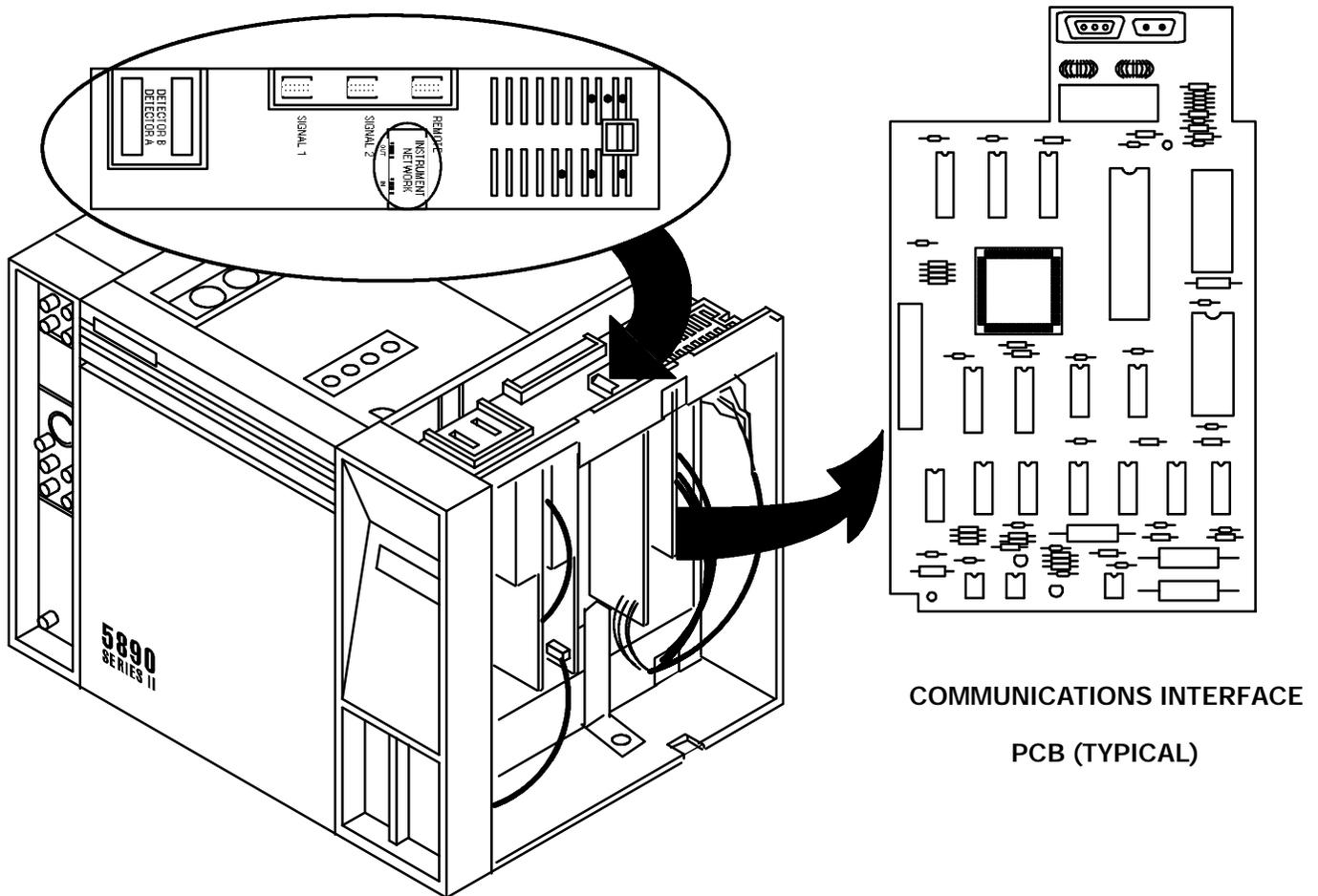
12. Install the replacement PCB by inserting it straight into its connector on the main PCB.
