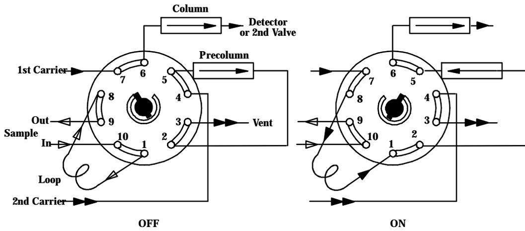
Gas Sampling with Backflush of Precolumn to Vent, Option 401 or 431
