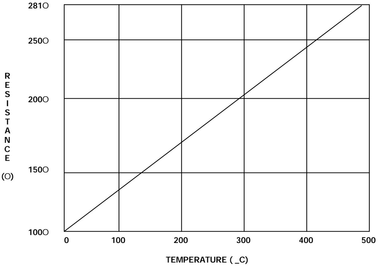
TEMPERATURE SENSOR RESISTANCE VS. TEMPERATURE
