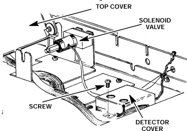
6. If the detector is not going to be replaced with a new detector, cap the detector base.
