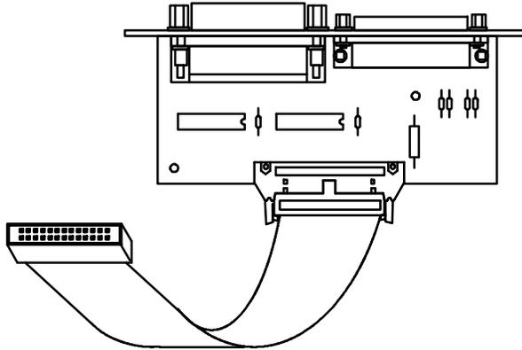
11. Free and remove the ribbon cable from the rear panel connector PCB by releasing the locking tabs (one on either side of the connector receptacle) and pulling the cable straight out.
