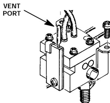
6. Cap the TCD vent port on the top of the detector. (This is not be required on a series connected TCD.)
