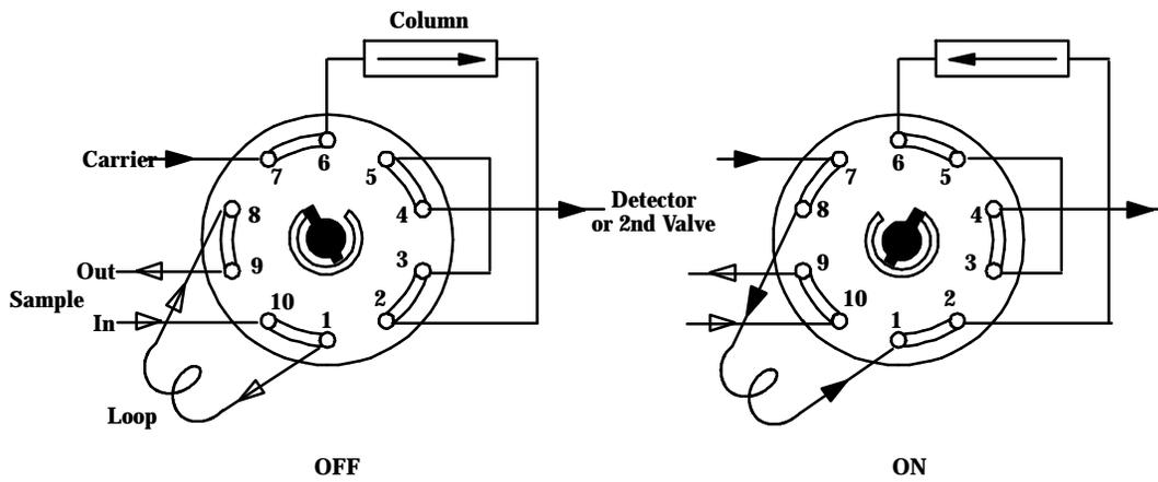
Gas Sampling with Backflush to Detector, Option 402 or 432
