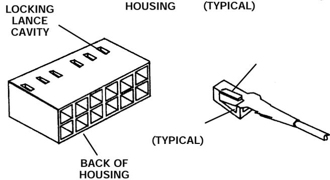
26. Insert the plug in its receptacle (P8) on the main PCB. (The plug is keyed and can only be inserted one way.)
