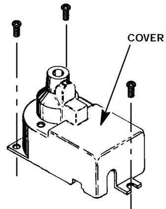
10. Use a Pozidriv screwdriver to remove the three screws securing the detector cover to the thermal strap.
