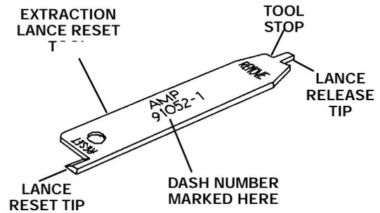
23. Prepare the pins corresponding to the replacement stepper motor by adjusting their locking lances using the lance reset portion of the tool.
