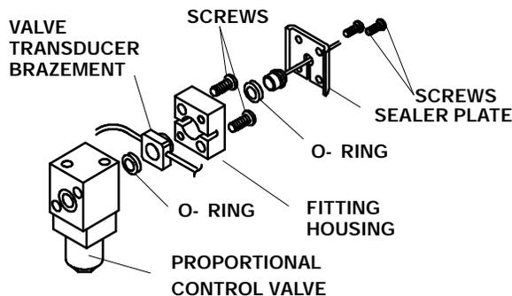
22. Remove the two screws securing the fitting housing to the proportional control. (This will free the valve transducer brazement from the proportional control valve.)
