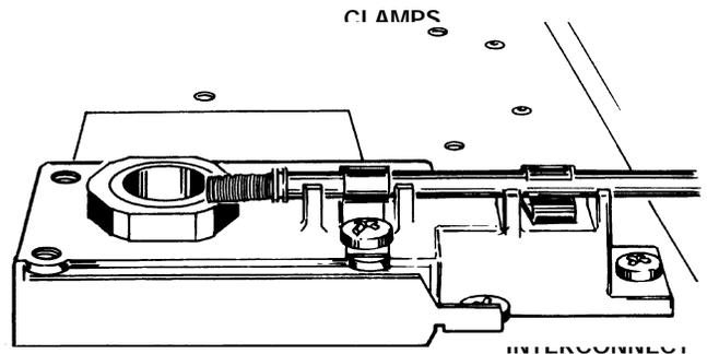
54. Tighten the screws on the clamps which secure the interconnect to the thermal strap.
