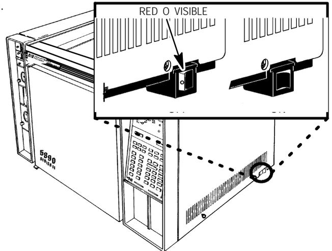
6. Remove the electronics carrier top cover by grasping it at the rear and lifting until its catch releases, then pulling it toward the rear of the instrument.
