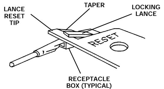
22. Insert the pins for the replacement sensor into their appropriate locations in the plug, making sure the locking lance on each pin seats into its hole through the side of the plug.
