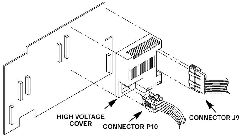
13. Remove the high voltage cover from the upper right portion of the main PCB.
