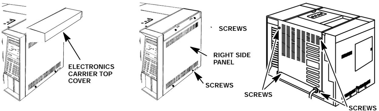
9. Remove the four screws securing the rear cover at its upper rear portion.
