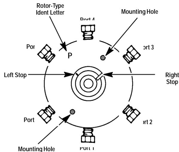
The valve body is made of Nitronic- 60. This is a high chromium, high nickel content stainless steel, that has excellent chemical resistance, anti galling characteristics, and high tensile strength. External tubing (plumbing) is connected to the valve body ports by the use of provided ferrules and fittings.
