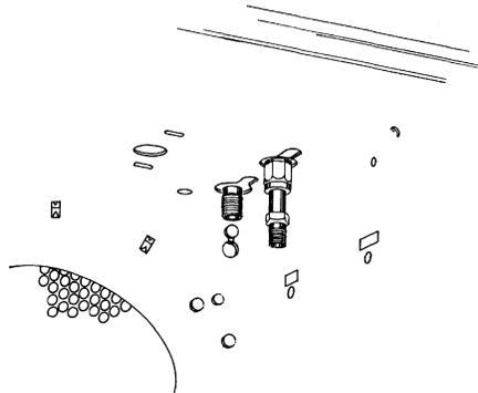
13. Use a 1/4- inch nut driver to remove the jet from the detector weldment.
