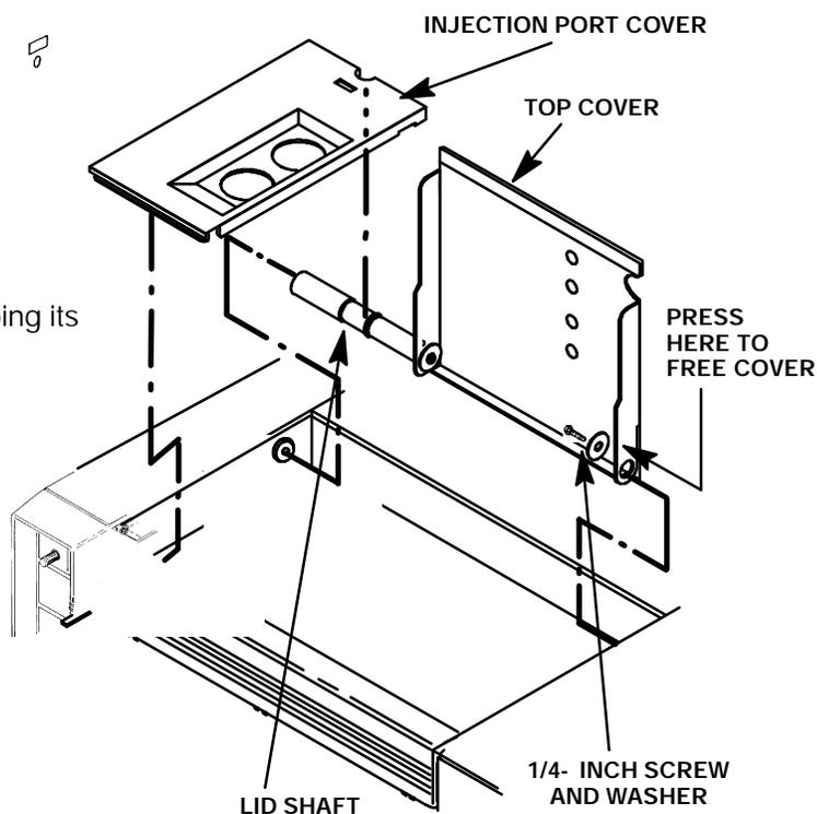
10. Remove the screw securing the ground strap to the hinged top cover
