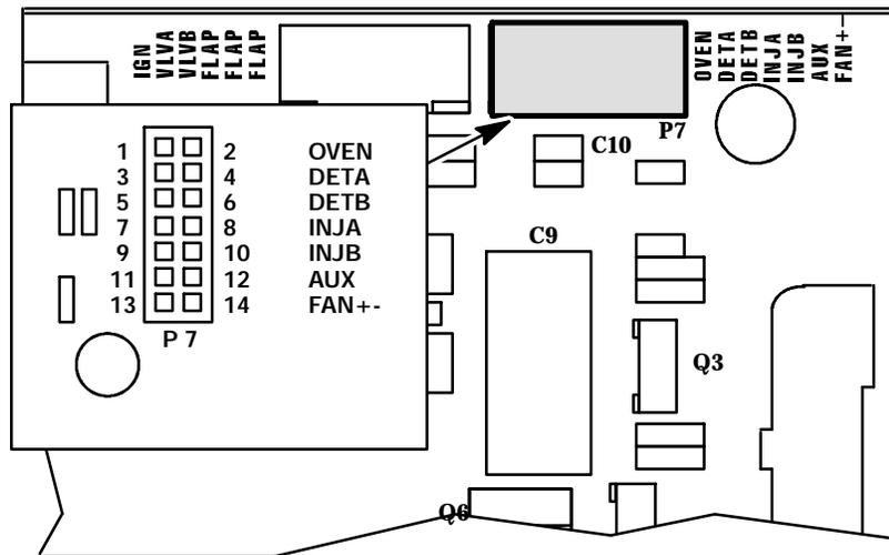
22. Use the lance release tip of an AMP pin extraction/lance reset tool (8710- 1542) to remove the appropriate pins from connector P7. (The tool features a lance release tip and a lance reset tip. The lance release tip is used to depress the pin locking lance to extract the pin from a connector. The lance reset tip positions a locking lance to its proper height to ensure retention of the pin in the connector.)
