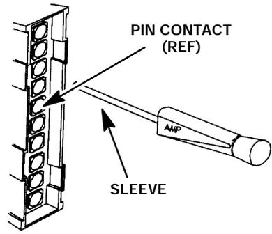
25. Insert pins from the new valve into their appropriate locations in the plug, making sure the locking lance on each pin seats into the plug.
