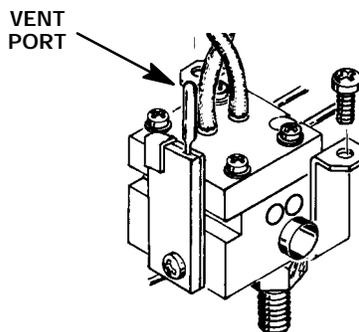
11. Disconnect the detector filament and delta-temperature sensor leads at their connector block on the detector PCB. Use a small flat-blade screwdriver to press each wire lead release (located adjacent to each connection).
