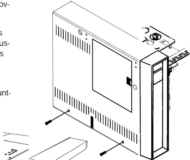
13. Remove the two screws securing the left side panel along its bottom edge.
