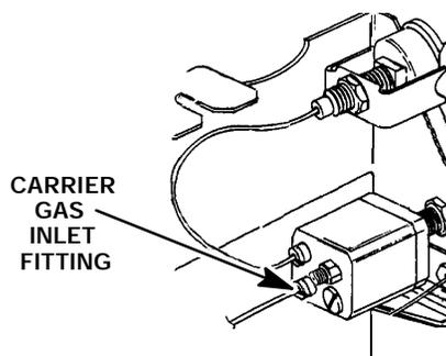
11. Remove any insulation from around the top of the inlet.
