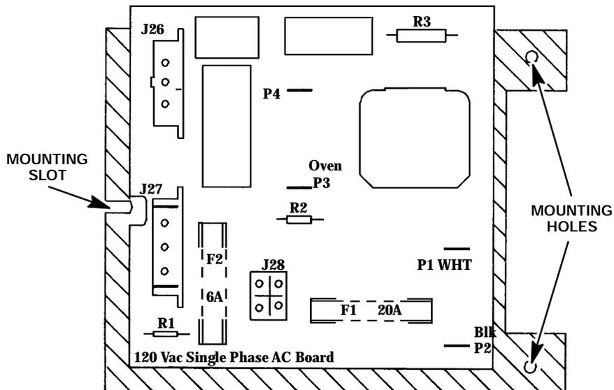
14. Install the replacement AC power supply PCB in the reverse manner by sliding the mounting slot on the left side of the PCB mounting bracket under the loosened mounting screw adjacent to the transformer.
