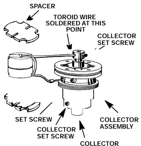
8. Use needle- nose pliers, inserted through the opening in the top of the detector cover, to remove the collector by forcing it down from inside the top of the collector assembly.
