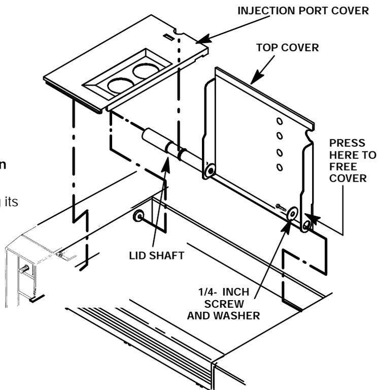
10. At the lower right edge of the cover, press from right- to- left until the right side hinge releases.
