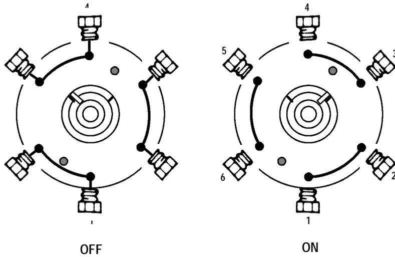
Above is illustrated an actual 6 port valve viewed from the actuator side. A functional two dimensional diagram representing the same valve is shown.
