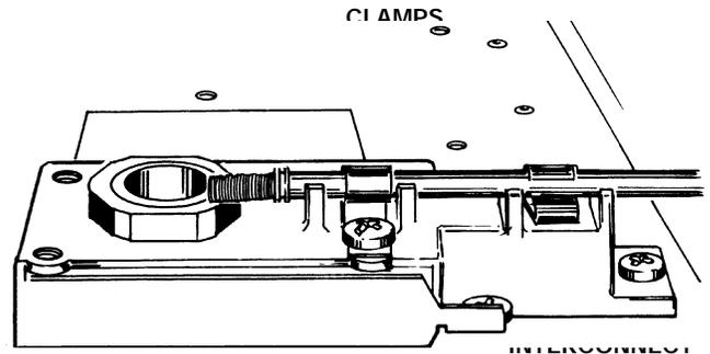
53. Tighten the screws on the clamps which secure the interconnect to the thermal strap.
