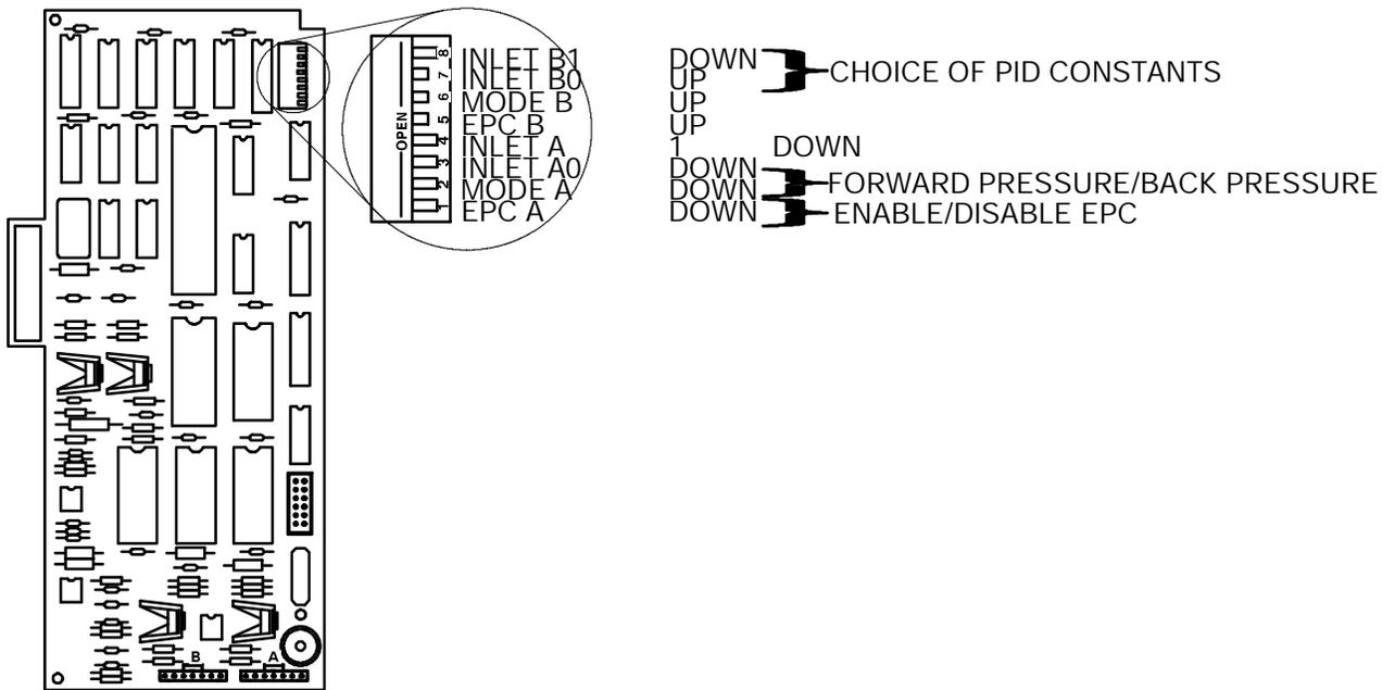
TYPICAL SWITCH SETTINGS FOR EPC/MPC PCBs
