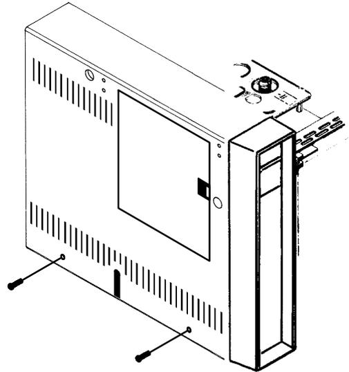
13. Remove the two screws securing the left side panel along its bottom edge.
