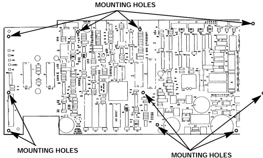
13. Remove seven screws securing the main PCB to the electronics flow carrier.
