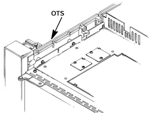
20. Bend the tube running from the installed inlet to the inlet flow control components so that it lays within the "U"-shaped channels to the left of the inlet.
