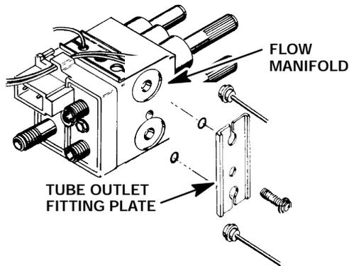
34. Disconnect the tubes by removing the tube outlet fitting plate from the manifold block.
