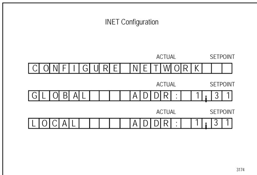
Figure 13-4. “CONFIGURE NETWORK” Displays
