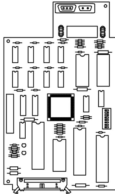
16. Install the ribbon cable into the connector receptacle on the rear panel connector PCB. (When the connector is properly seated, the locking tabs on the connector receptacle will wrap around the edge of the connector, locking it in place.)
