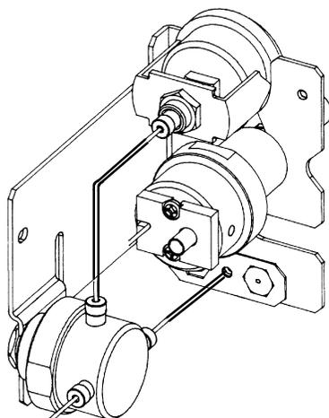
8. Remove two nuts securing the flow module to the mainframe (one next to the pressure gauge, and one at the lower edge of the module).
