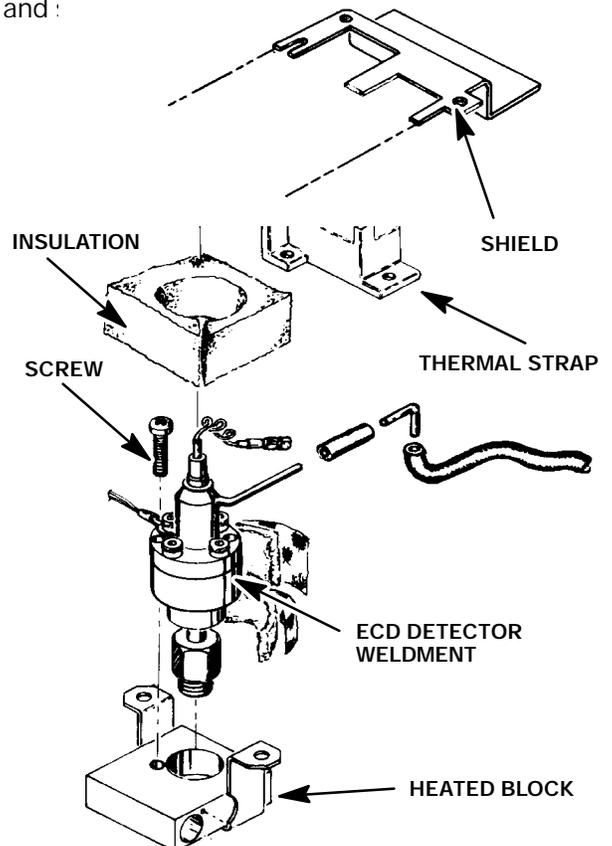
17. Remove the thermal strap, working it carefully over the collector lead and exhaust vent tube.
