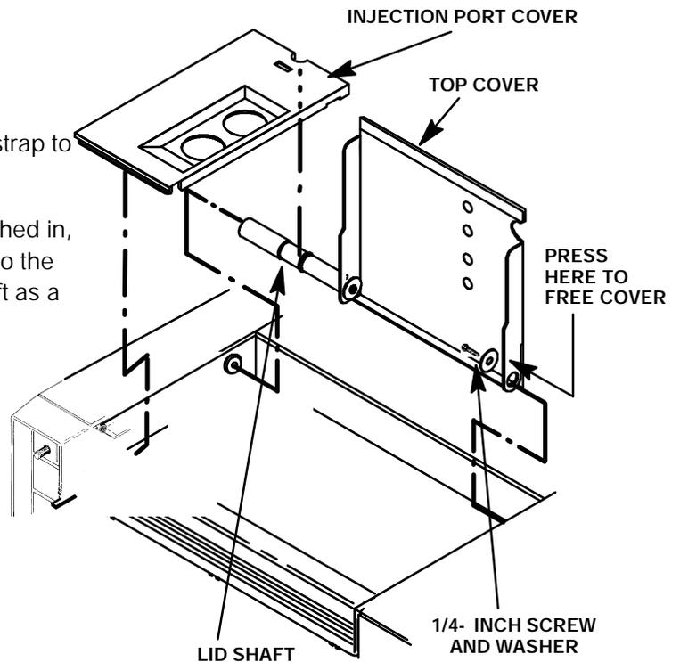
9. Using a Pozidriv screwdriver, remove the screw securing the detector top cover to the thermal strap.
