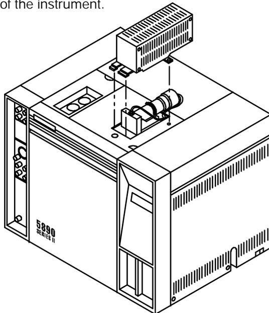
8. Lift the detector top cover to expose the FPD detector weldment.
