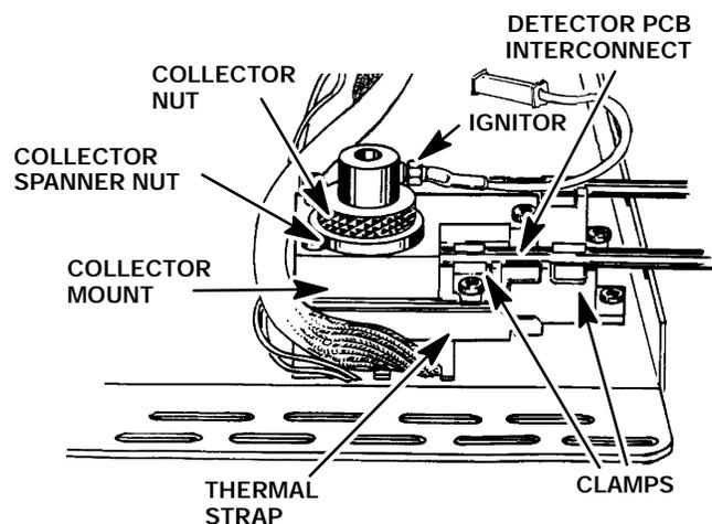
6. Use a wrench to remove the ignitor from the FID ignitor castle.
