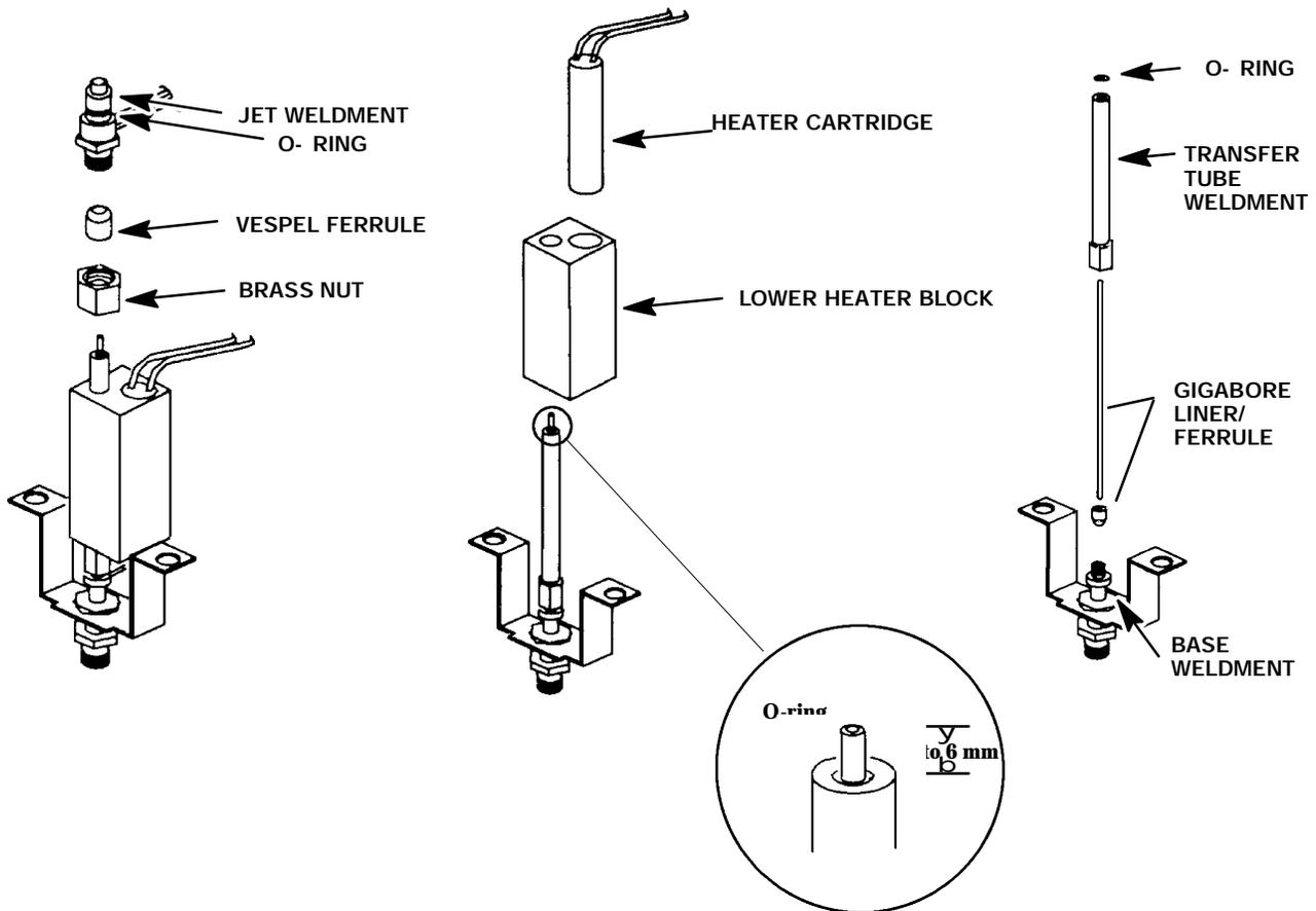
21. Unscrew the transfer tube weldment from the detector base weldment.
