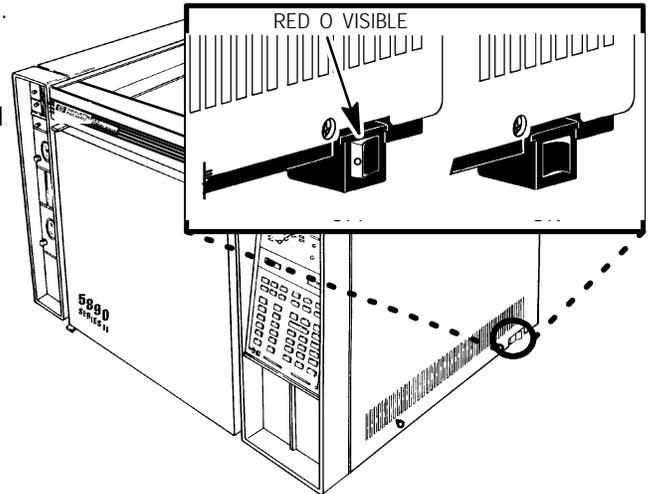
6. Slide the rear cover towards the rear of the instrument.
