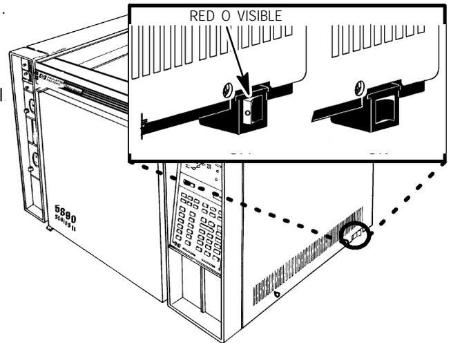
6. Remove the rear cover by sliding it towards the rear of the instrument.
