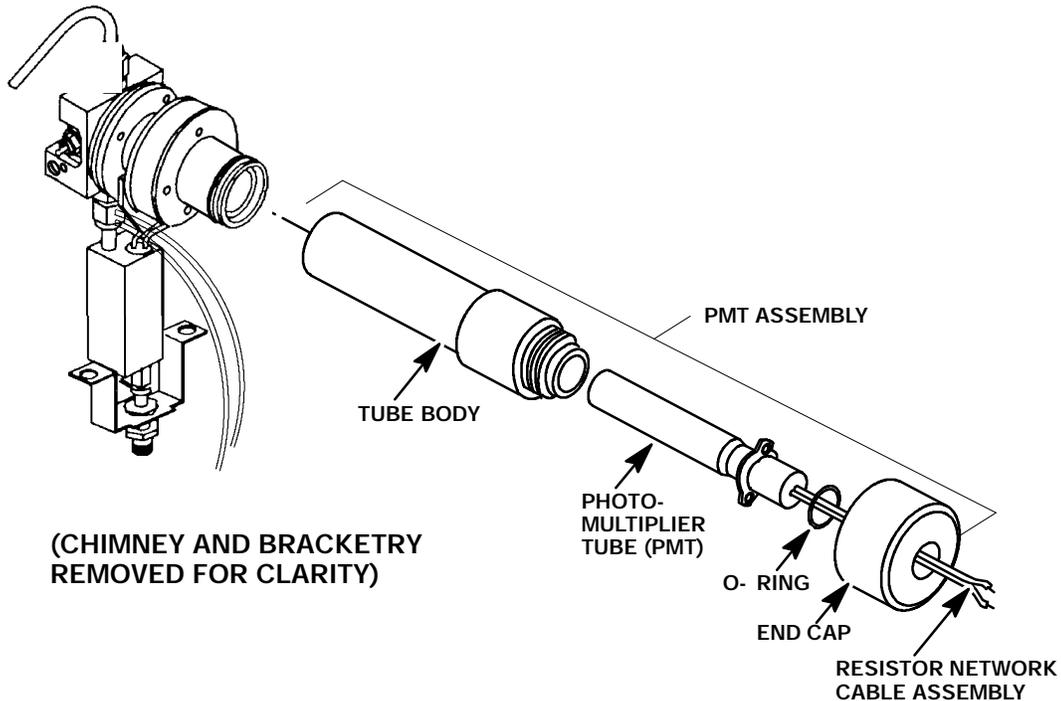
10. If the PMT is not to be replaced, clean the window of the tube with a lint- free lens tissue and proceed to step 15 . (If necessary clean the window with a solution of soft soap and warm water. Rinse with distilled water.)
