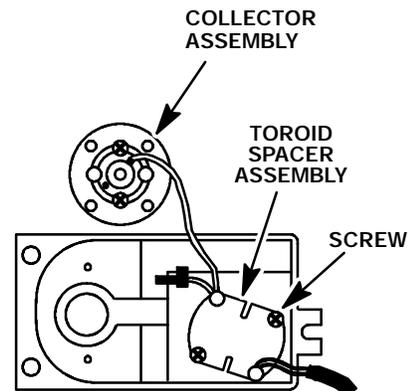
17. Remove the collector assembly and the toroid spacer assembly from the detector cover, as a unit.
