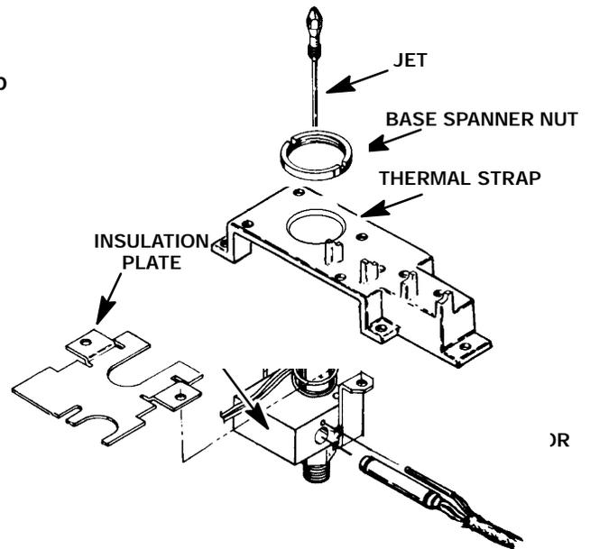
38. Install the insulation around the detector weldment.
